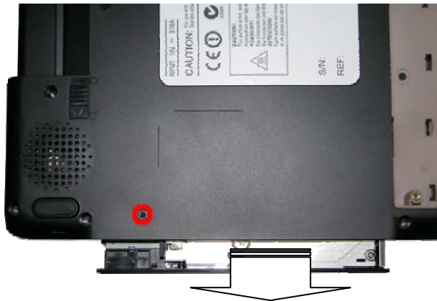
Fig. 6 Removing the optical drive
